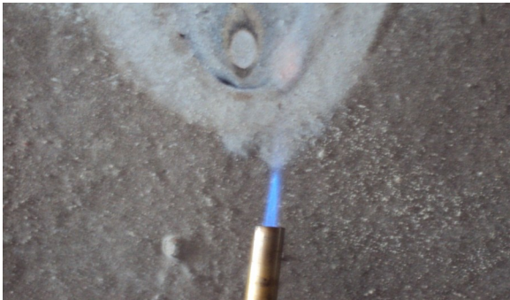
-Tested at 3600 degrees with a propane blow torch
